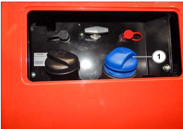
Figure 122: Filling the "DEF" tank
