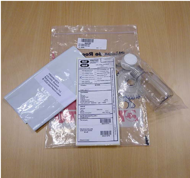
Figure 173: Hydraulic oil contamination check
